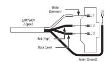
Ensure wiring circuit agrees with diagram and leads are securely tight.
